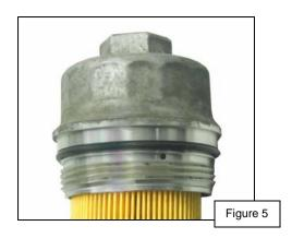
Always use caution when installing any oil filter housing o-ring. The threads on the caps can be sharp and may cut into the o-ring. This can compromise the o-ring and cause it to fail. The result is oil loss and potential catastrophic engine failure.
