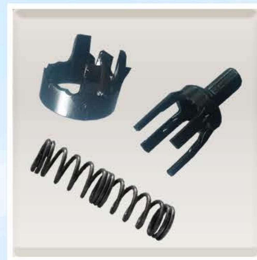
Broken Oil Bypass Valve Components
